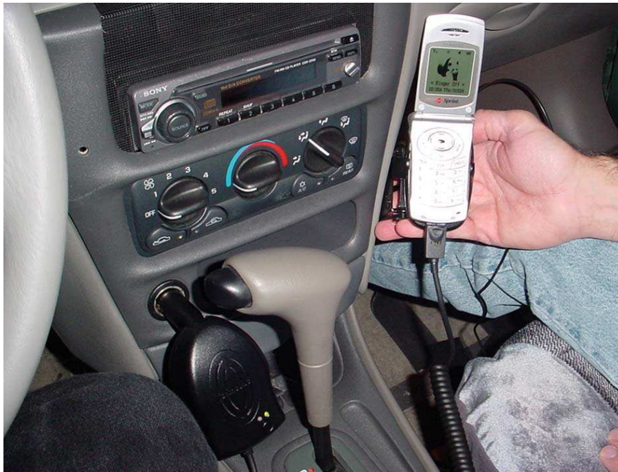
Figure 13. Photograph Showing VSHF Hands-Free Speaker Kit Setup and Phone Cradle Location.
