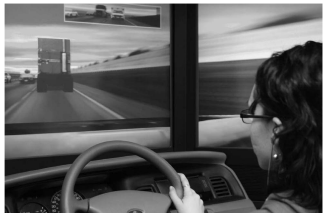
Figure 1. PatrolSim driving simulator used in the experiment.
