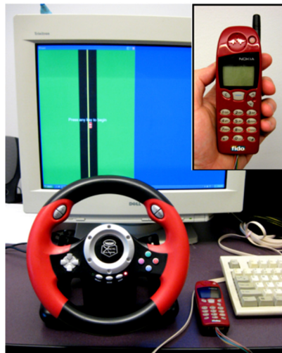
Fig. 1. Apparatus including the monitor, steering wheel, keyboard, and mobile phone. Inset: Close-up of the mobile phone used in the experiment.
