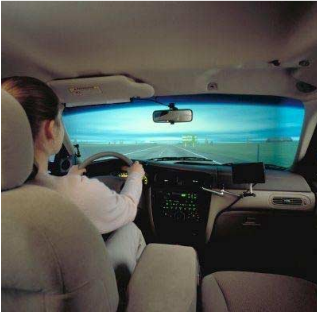
Figure 2 The Taurus cab mounted inside VIRTTEX
