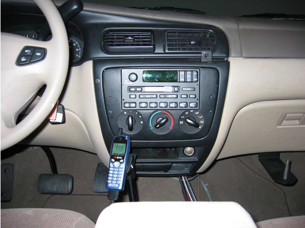
Figure 5 Radio, climate-control and hand-held phone locations. Drivers removed the phone from its holder during use.
